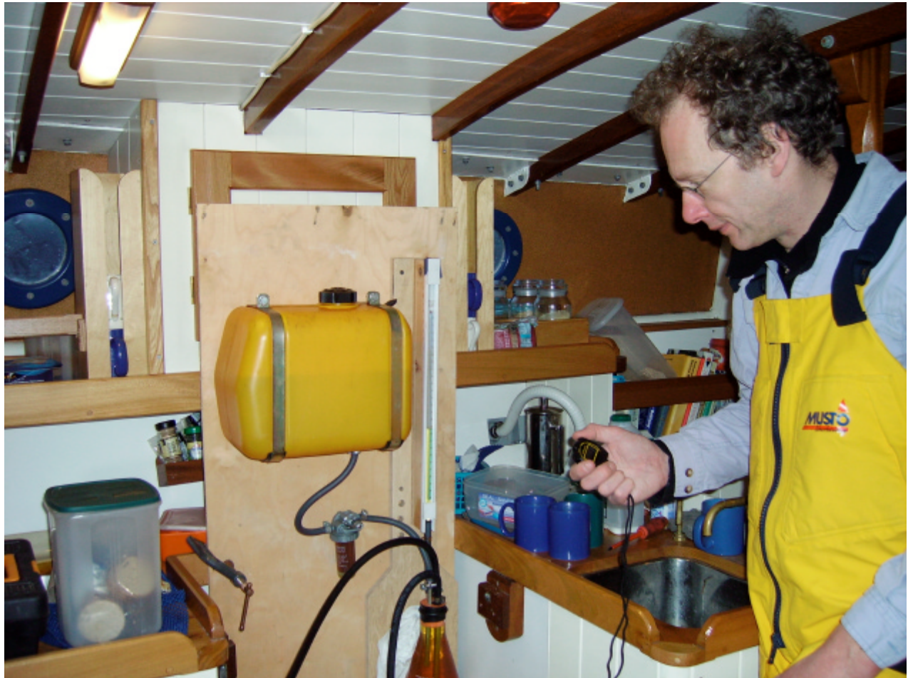
Plate2, measuring fuel consumption on "Apple"
